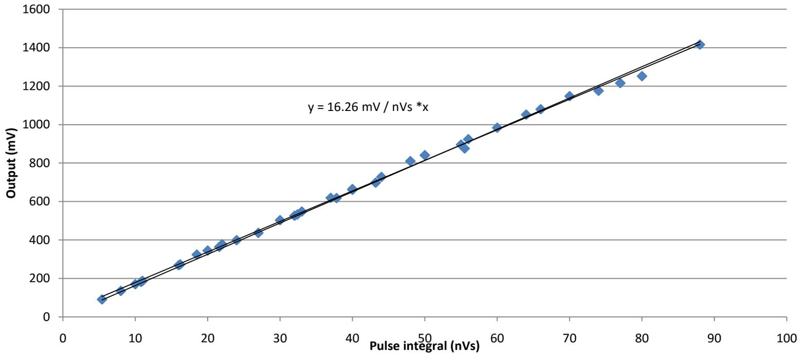
Choose PMT gain so expected signal sums to  $\sim 60$  nVs giving  $\sim 1$  V output. Discriminate at eg.  $\sim 0.25$  V.
