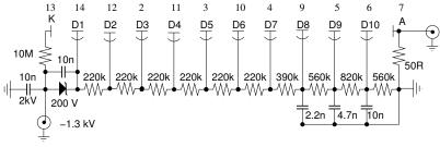
Resistors 0.330W, 150V 200ppm/C Vmax 1.5kV Imax 0.35 mA
