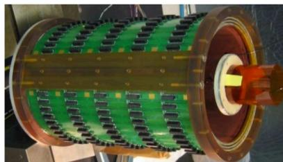
Figure 15: (left) Photograph of the BoNuS RTPC, showing the left module with the readout padboard removed and a complementary exploded view exposing the components of the right module. (right) Photograph of the eg6 RTPC during assembly.
