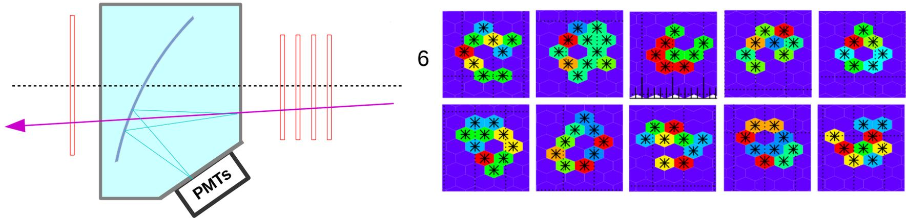
Light generated by particles will be reflected to the PMT matrix, and leave signal such as the ones seen above (right).
