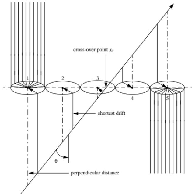
Fit to  $n_{avg} \approx 5$  independent time measurements per plane yields a position resolution of  $\approx 225 \mu\text{m}$  FWHM
