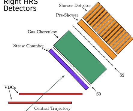
FIG. 1. Configuration of HRS detectors as used in Experiment E12-07-108.
