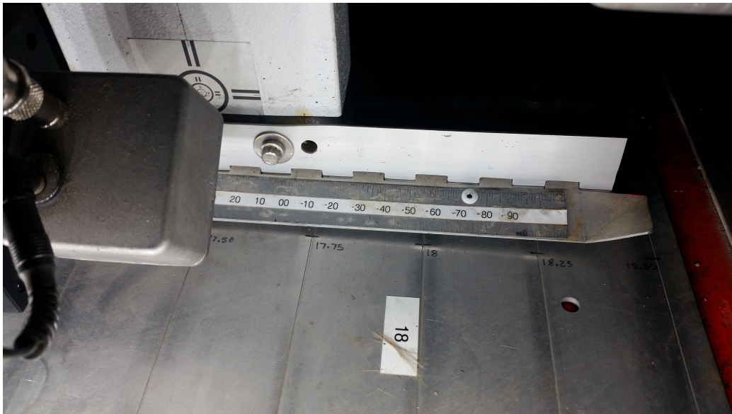
Figure 3: Photo of Left HRS angle system. The more negative vernier values correspond to larger floor mark angles, in agreement with the equation in the text.
