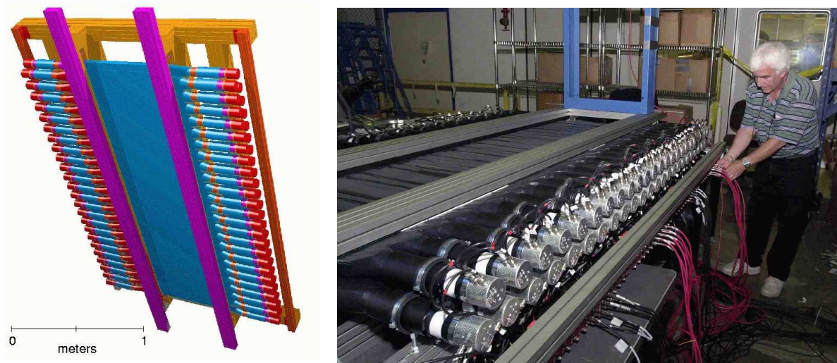
Fig. 14. Scintillation counters used for the BigBite trigger \Delta E/E detectors
