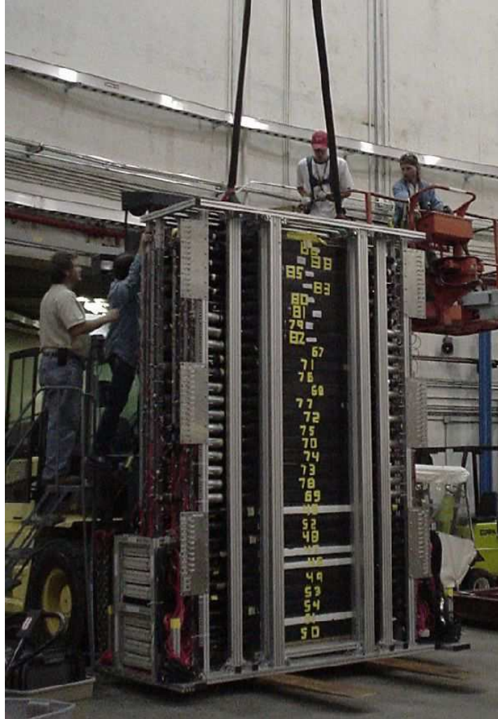
Figure 4: Shown is the Hall A Neutron Detector (HAND). This device has been successfully used in Hall A and is being prepared for the upcoming ^3\text{He}(e,e'\text{N}) experiment (E05-102).
