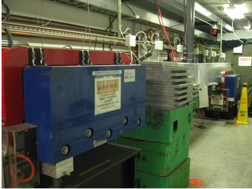
Figure 4.9: The upstream half of the Compton chicane in the Hall A tunnel, looking downstream. The blue return yoke and red coil of the first dipole are visible at left; at right is the second dipole and the laser table (behind an olive-green curtain).
