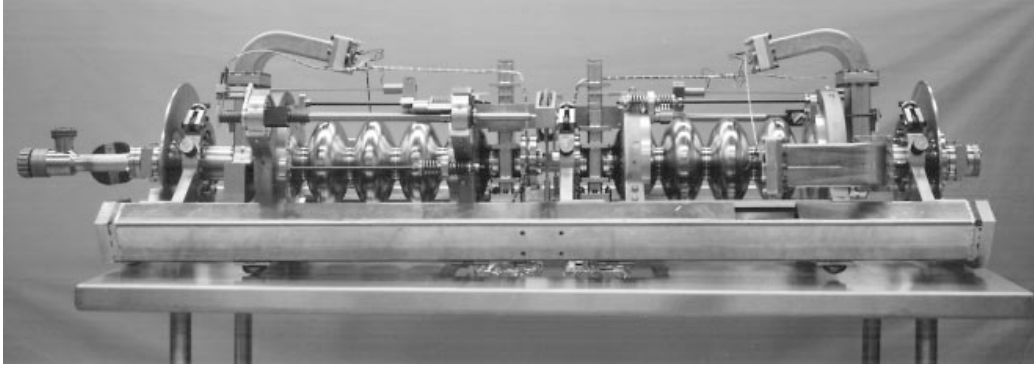
Figure 3.7: Pair of accelerating cavities, later installed in the CEBAF beamline. Each 50-cm cavity contains five cells. Four cavity pairs make up a cryomodule. Reproduced from Leemann et al. [130].
