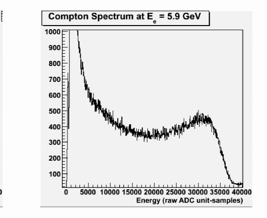
Planned upgrade to a green Compton laser (double the incident photon energy) will give us access to more of the spectrum at one-pass
