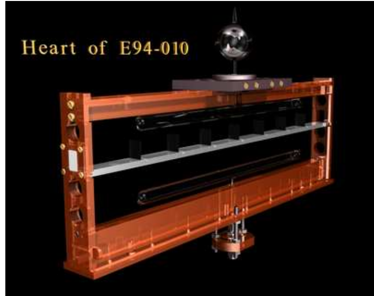
Figure 2.16: Target ladder containing the main polarized target cell (top), the seven ^{12}\text{C} foils (center middle), the BeO target window (front middle), and the reference cell (bottom).
