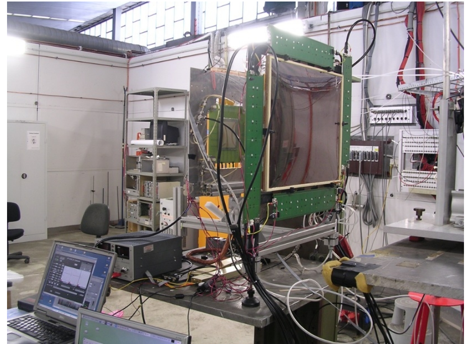
Stretching GEM foil on frame Reduced spacer material
