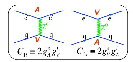
$$A_{PV} = \frac{\sigma_R - \sigma_L}{\sigma_R + \sigma_L} \sim \frac{\tilde{A}_Z}{A_\gamma} \sim \frac{G_F Q^2}{4\pi\alpha} (g_A^e g_V^T + \beta g_V^e g_A^T)$$
