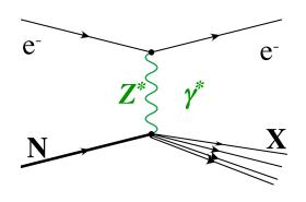
$$A_{PV} = \frac{G_F Q^2}{\sqrt{2}\pi\alpha} \left[ \mathbf{a}(x) + Y(y) \mathbf{b}(x) \right]$$
