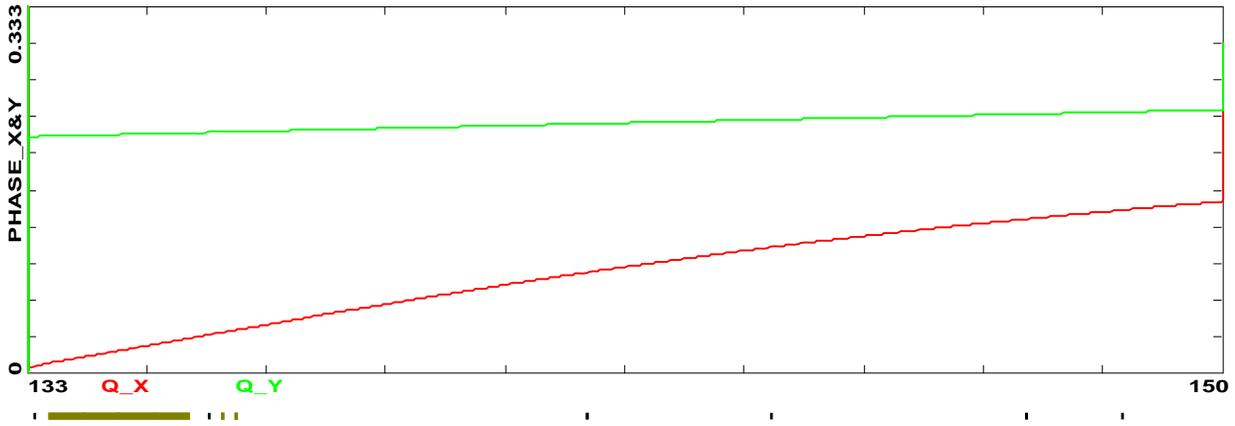
Figure 7. Phase advance from start of fast raster. Vertical axis 0 to  $2\pi/3$ . If more phase advance is desired, the Moller quads may be used. Compromise with beam size at target is necessary.
