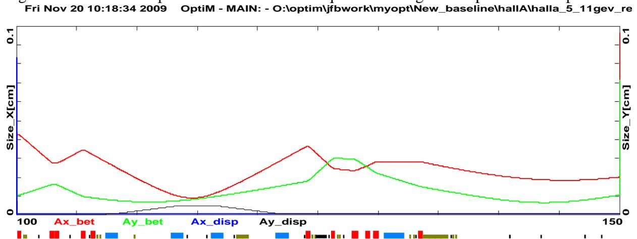
Figure 15. Beam envelope for region in Figure 14. 1mm vertical scale. Beam elliptical at pivot.
