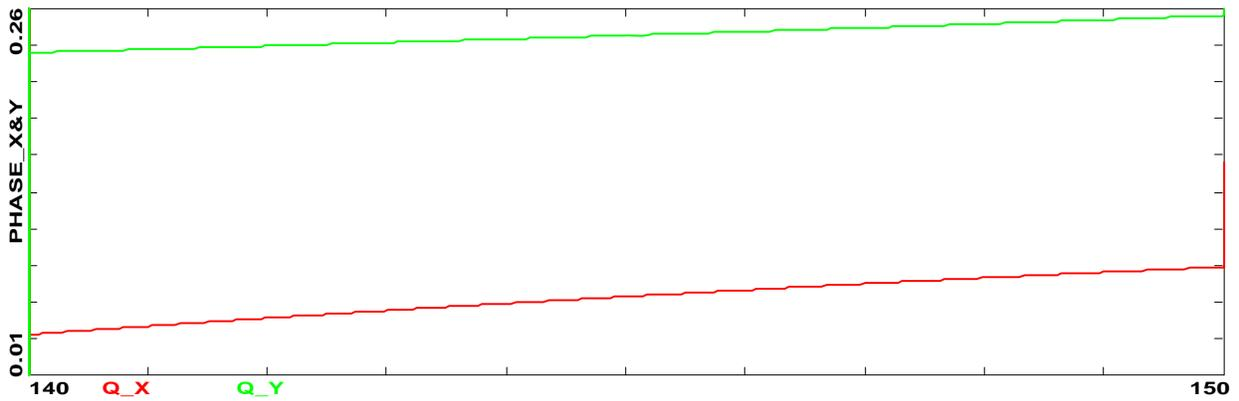
Figure 10. Phase advance between the last pair of BPMs. They are tick marks  $\sim 141\text{m}$  and  $\sim 147\text{m}$ . Note change of vertical axis vs figure 7. Vertical axis  $\pi/2$  extent. Vertical phase advance about six degrees and horizontal about ten degrees.
