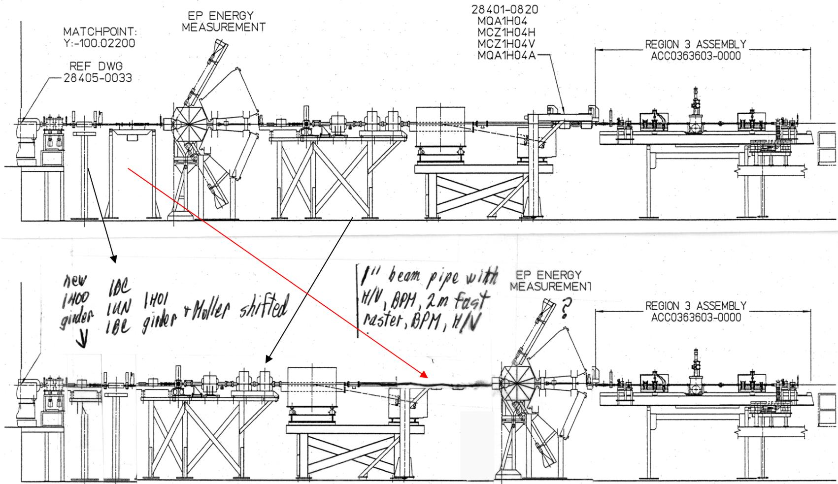
Old and new beamlines from end of Compton to pivot. Only 4.5m is available where the ep system is shown in the new beamline.
