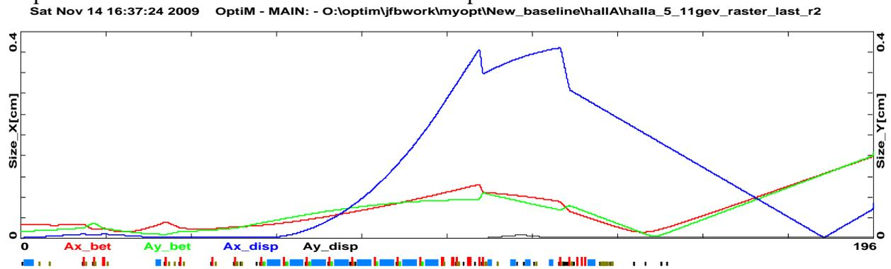
Figure 13. Beam envelopes corresponding to figure 12. Vertical axis 4mm. Dispersive term in blue again.
