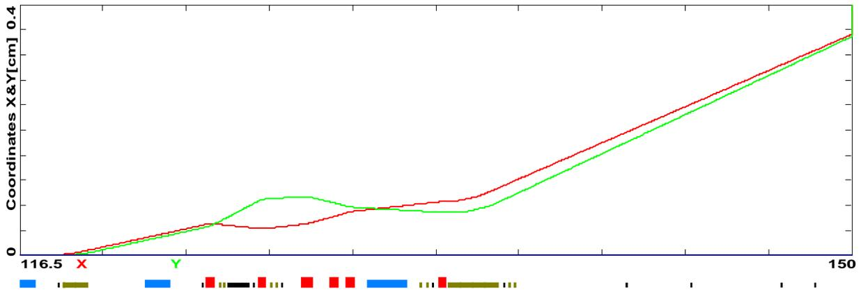
Figure 18. Existing fast raster moved to final leg of Compton chicane to provide raster for high current Moller target. Target raster also on at same field. These show DC kicks - raster phasing is important
