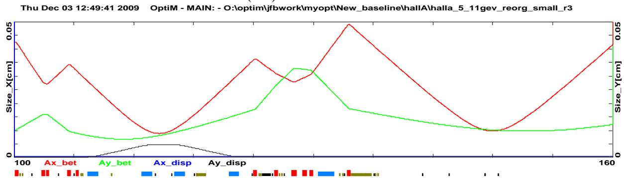
Figure 21. Beam envelope for optics above. Note that horizontal  $\sigma$  is  $0.5\text{mm}$  at the fast raster and  $0.1\text{mm}$  at the pivot. If the match can be accomplished  $\pm 20\sigma$  to tube wall in the raster is acceptable.
