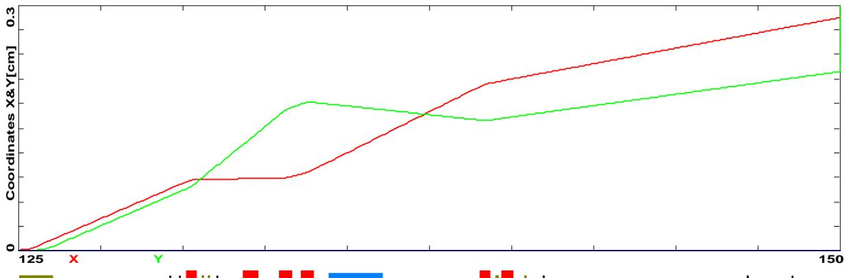
Figure 4. Fast raster excited at twice the 6 GeV maximum value. 3mm full scale. Pivot is 1.4m from the right vertical axis. No space is available to double the raster coil length due to eP.
