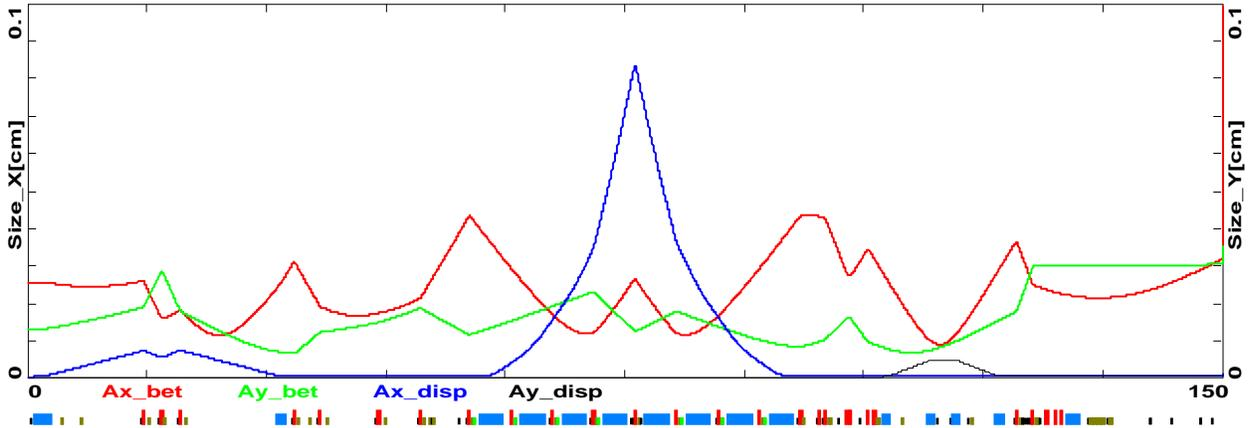
Figure 6. Beam envelopes, new design. If the Moller quads are turned on the beam size at the target will change and more phase advance may be obtained between the last pair of BPMs. Larger spot size is desirable per MOLLER collaborators.
