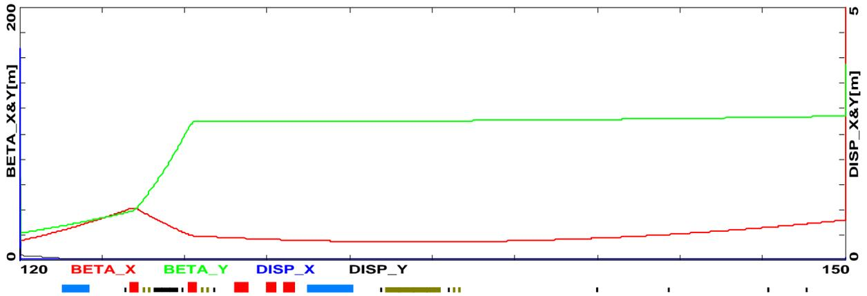
Figure 9. Beta functions starting near end of Compton chicane. One can more easily see here than in figure 5 that the Moller quads are turned off.
