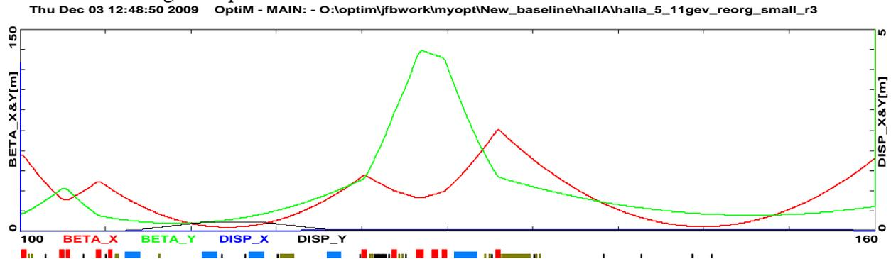
Figure 20. Betas for smaller spot at pivot. I show 10m more than in most of the figures so one can see how moving the minima via mismatch will change beam size. Pivot is  $\sim 149\text{m}$ , just before the minimum in the horizontal (red) curve.
