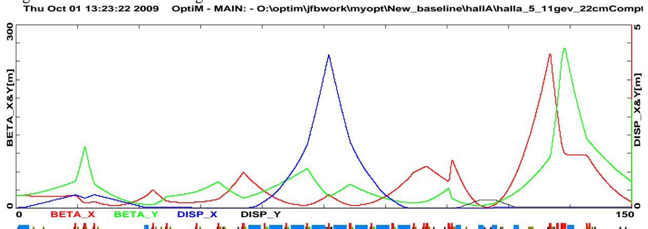
Figure 1. Betas and dispersion. Red horizontal beta, green vertical beta, blue horizontal dispersion, black vertical dispersion.
