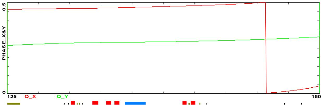
Figure 3. Phase advances starting at the fast raster. Very little vertical phase advance between the last two BPMs. Vertical scale is fraction of  $2\pi$
