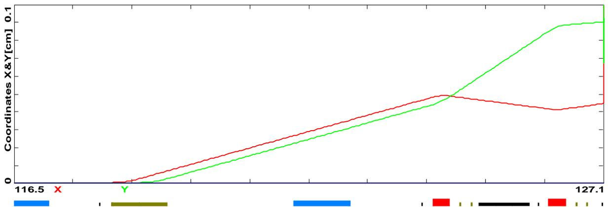
Figure 19. Enlargement of figure 18. Moller polarimeter target is at right end of plot. Vertical axis 1mm. Double these values for full raster pattern. Spot ~300 microns round at Moller polarimeter target - see figure 15.
