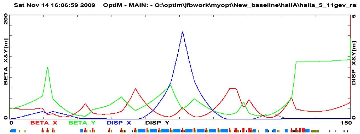
Figure 5. Betas and dispersion, new design. Only the quad doublet after the Compton is used in this plot. The Moller quads are turned off.
