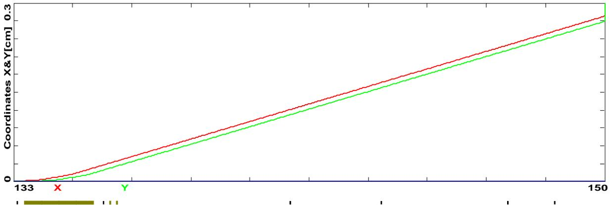
Figure 8. Fast raster excited at twice the 6 GeV maximum via twice the coil length. Coil length can't be doubled in the baseline design, so this design is easier to engineer than the baseline. 5mm square raster at the pivot. With the power supply implied in figure 4, the raster doubles that graphed.
