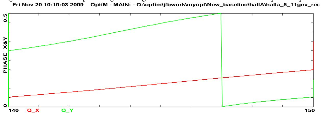
Figure 16. Phase advance, 180 degrees vertical scale. BPMs are at 140.7 and 147 m.
