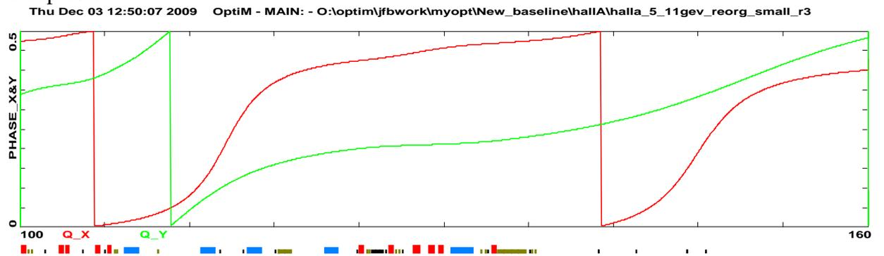
Figure 22. Phase advance for same region. Lots of phase advance for the BPMs at the end of the line.
