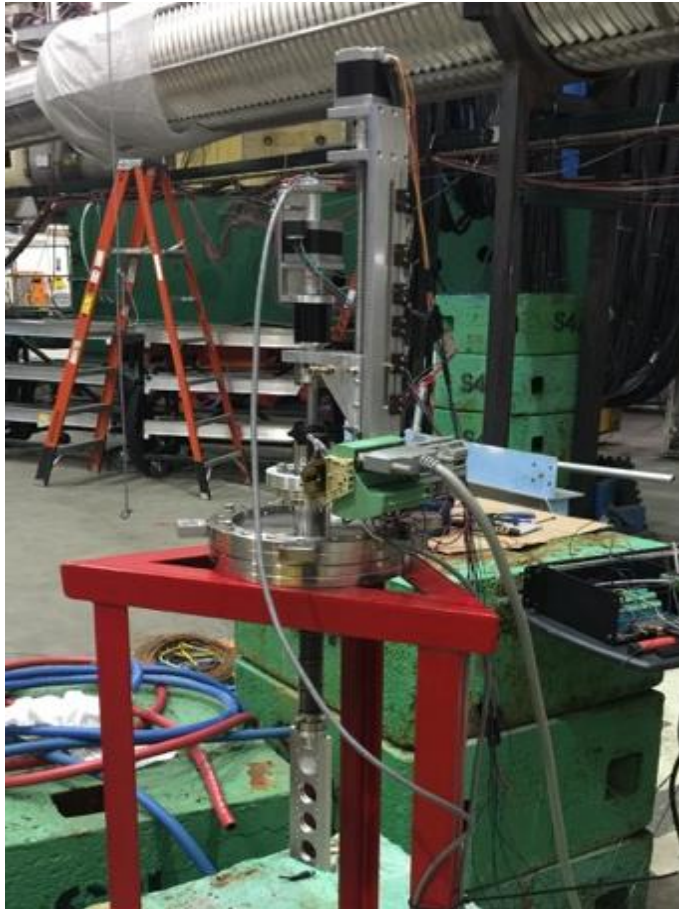
Figure 12: Target system. The target ladder with four foils installed can be seen at the bottom of the system.
