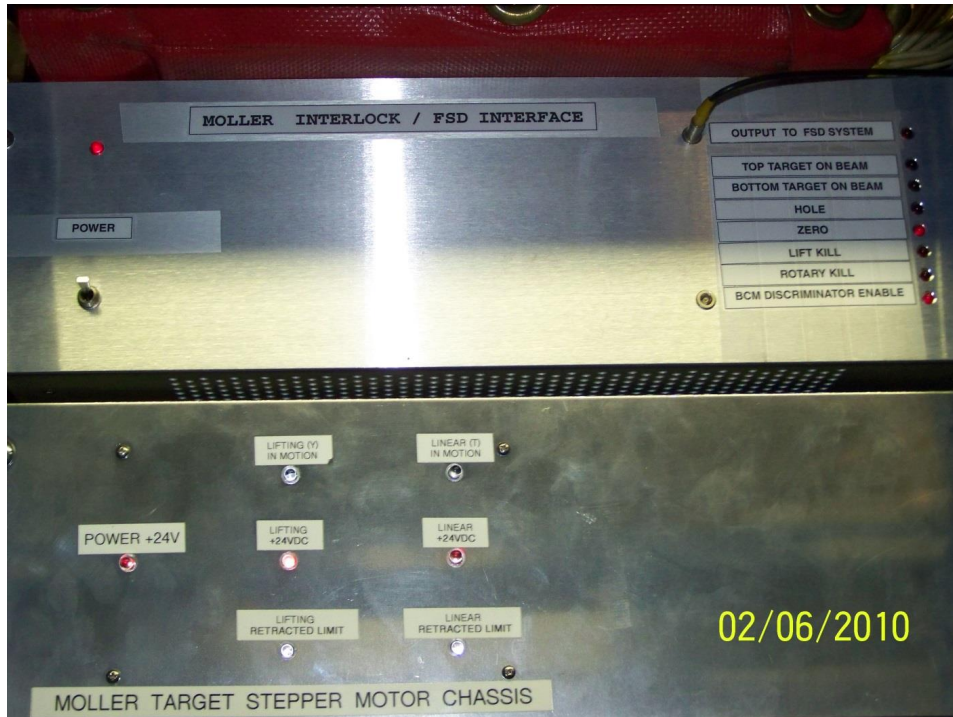
Figure 15: The Møller target motion may cause the Fast ShutDown (FSD) of the accelerator. The LEDs in the top right corner show the appropriate signals from the target. The top LED lit indicates no FSD signal.
