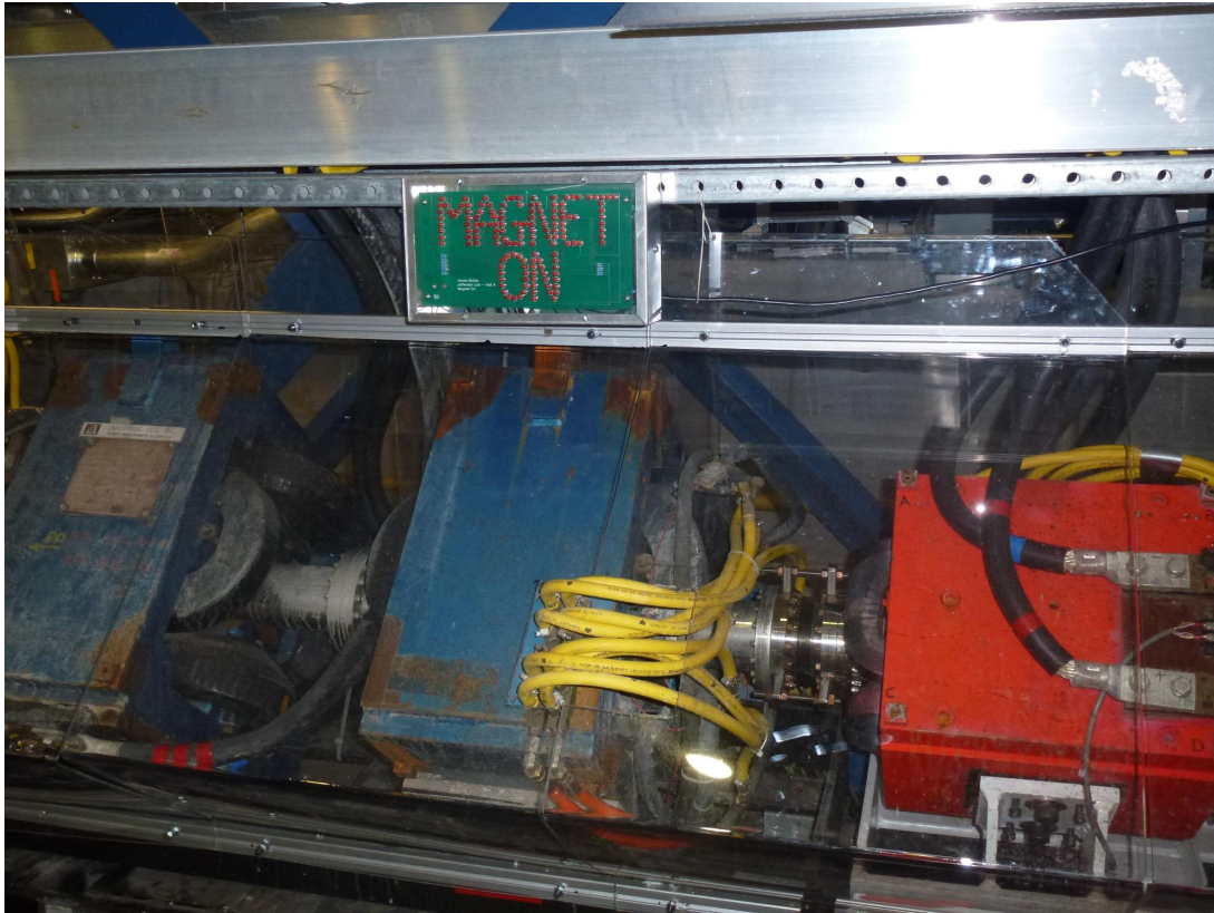
Figure 26: “MAGNET ON” light panel on the top of the Møller spectrometer shielding guard.
