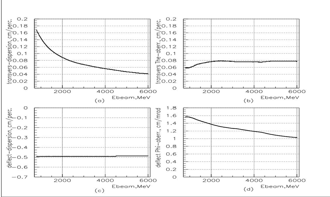
Fig.1,(a,c).The dispersion and  $\phi$ -angle aberration in deflective direction of the detector plane for beam energy range 1.0-6.0 Gev.
