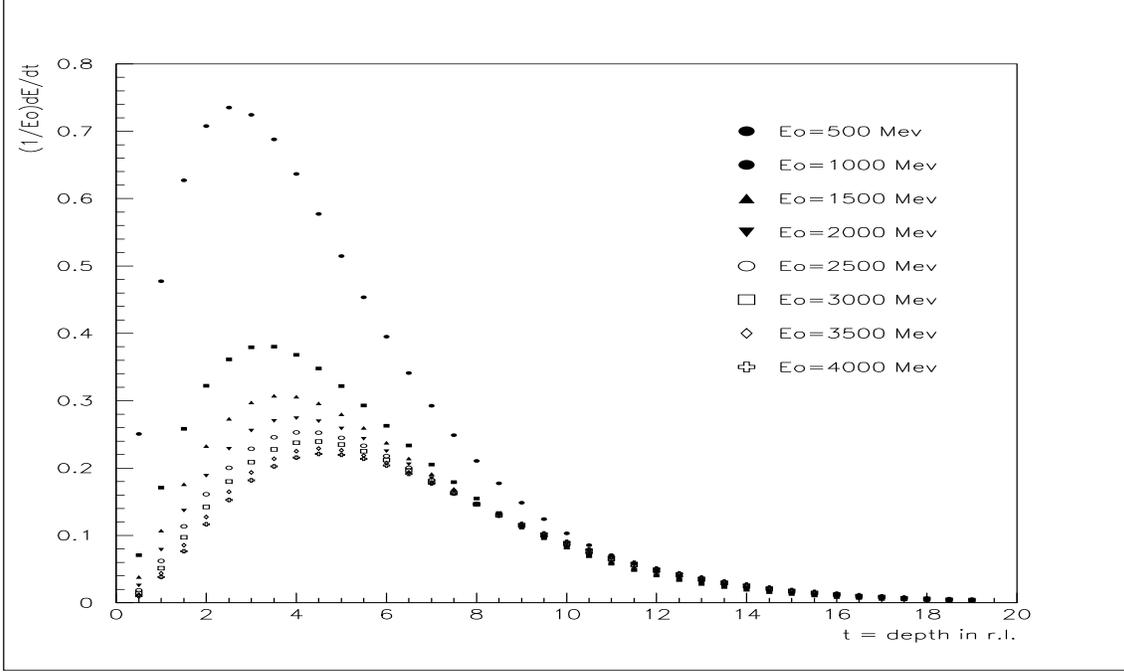
Fig.2. The energy deposition of electron induced shower for different particle energy in spaggetti-type material.
