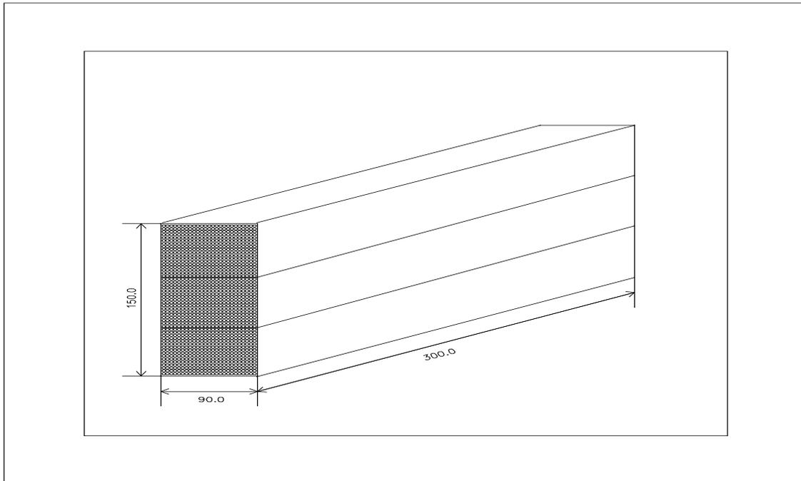
Fig.4. Schematic drawing of the construction of a single spaghetti-type module with three detector channels.
