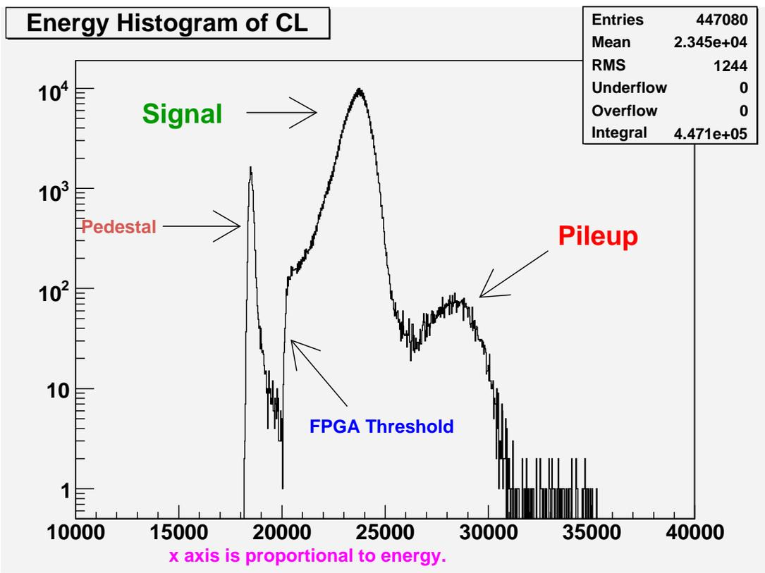
**FIGURE 2.** Integrated energy in one spectrometer from Møller calorimeters as processed by the FADC.
