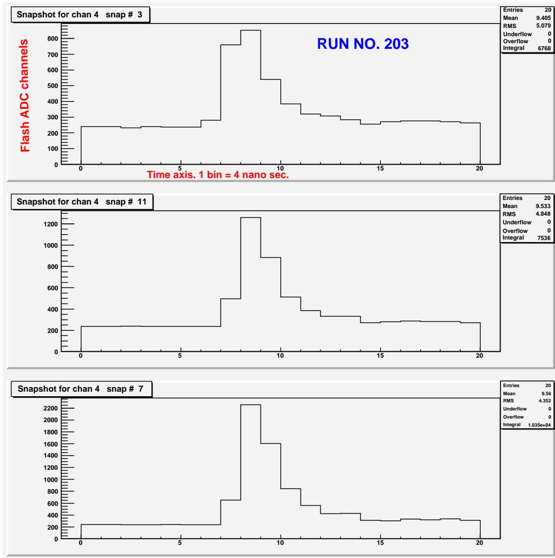
FIGURE 1. Typical pulses from the Møller calorimeter. Each snapshot shows the voltage versus time in the FADC.
