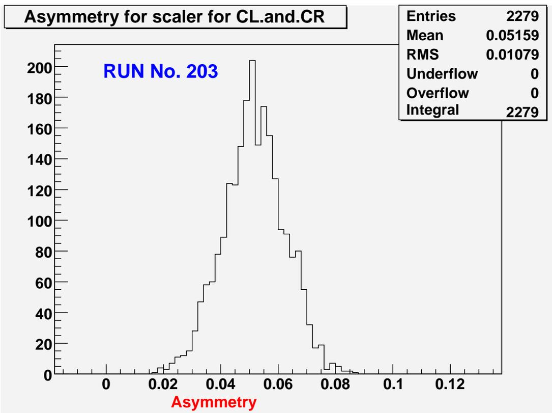
**FIGURE 3.** Møller asymmetry measured with on-board scalers in FADC. The 5% asymmetry is normal.
