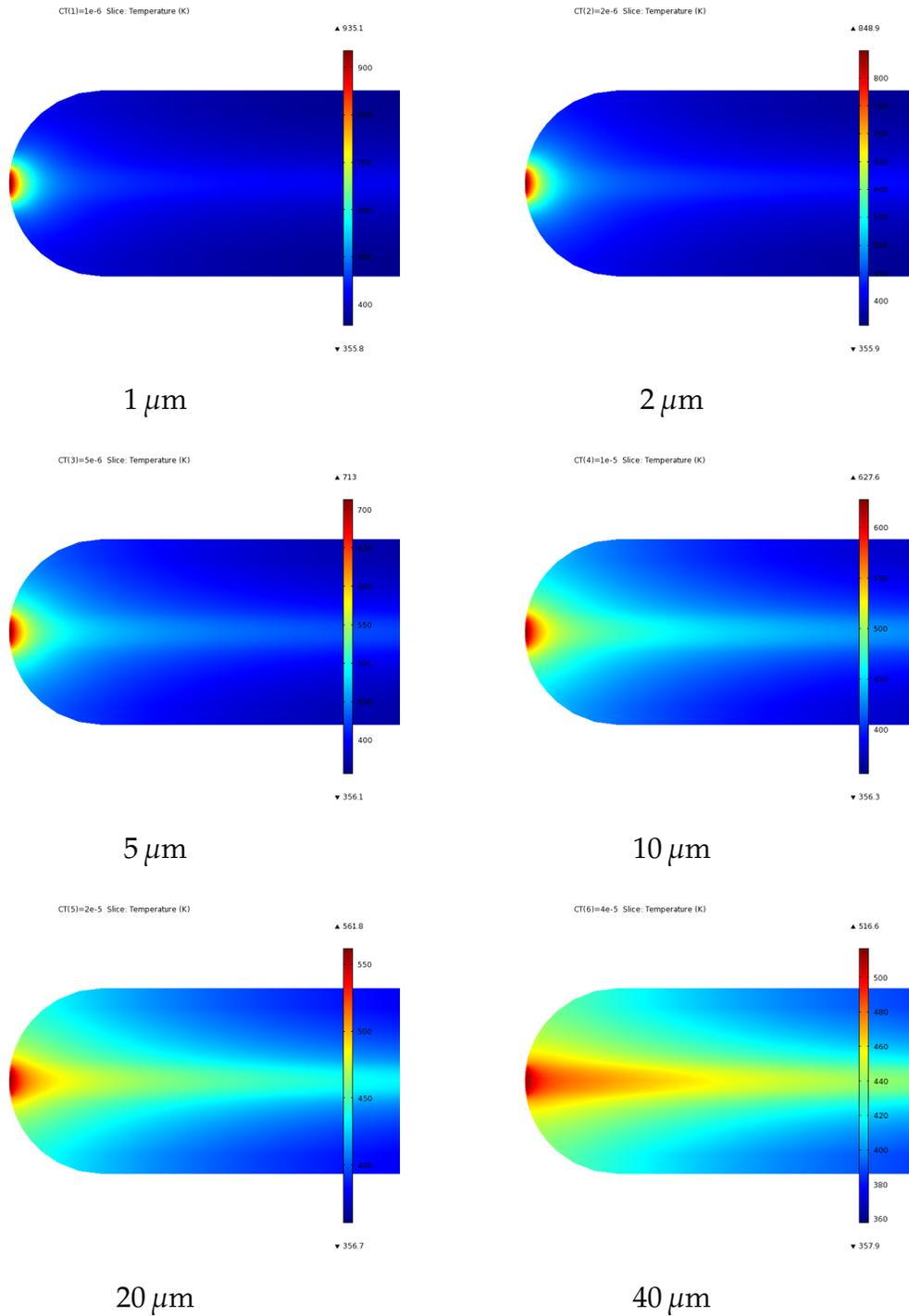
**Figure 7** Temperature distributions with copper coating, 30  $\mu\text{A}$
