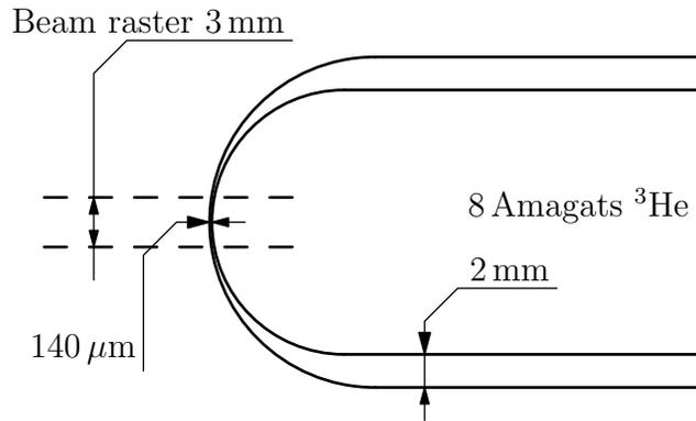
**Figure 2** Target cell, near the beam window
