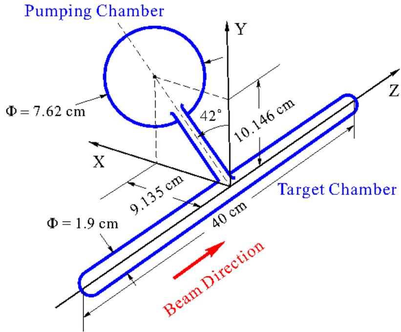
**Figure 1** The geometry of the target system
