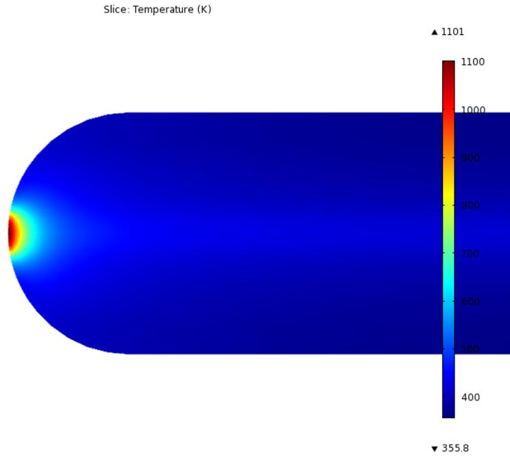
**Figure 6** Temperature distribution with  $30 \mu\text{A}$  beam current
