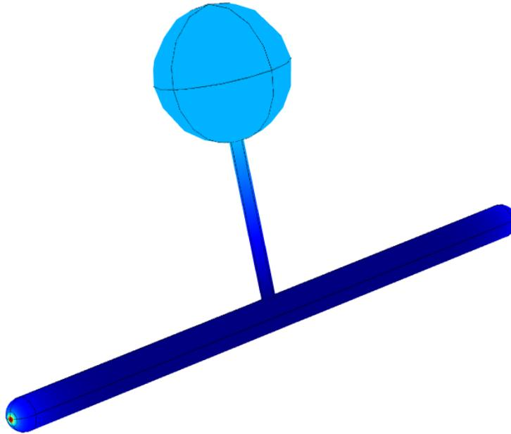
**Figure 4** Temperature distribution with  $12\ \mu\text{A}$  beam current
