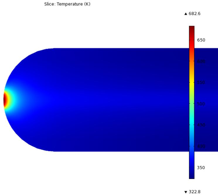
**Figure 5** Temperature distribution with  $12 \mu\text{A}$  beam current
