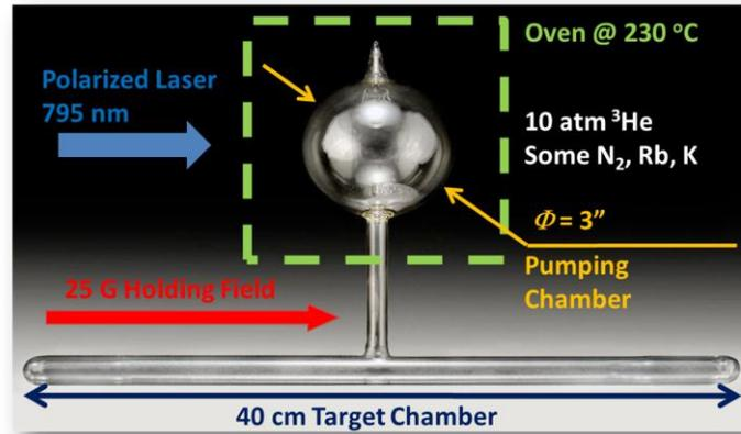
Fig. 5: Target Cell Conditions
