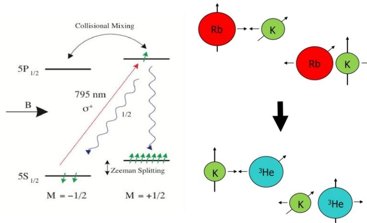
Fig. 3: Diagram of SEOP Process
