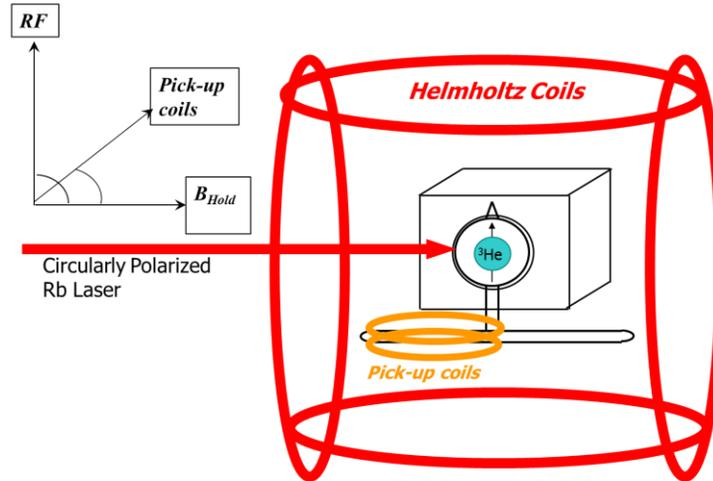
Fig.6: Target System Setup
