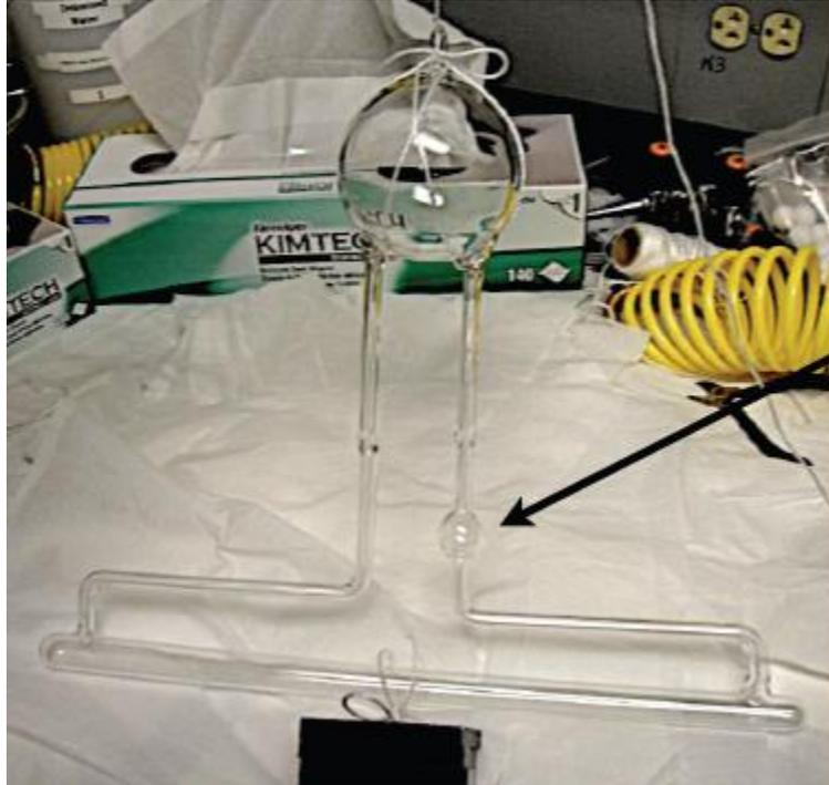
Fig. 2: New Convection Target Cell
