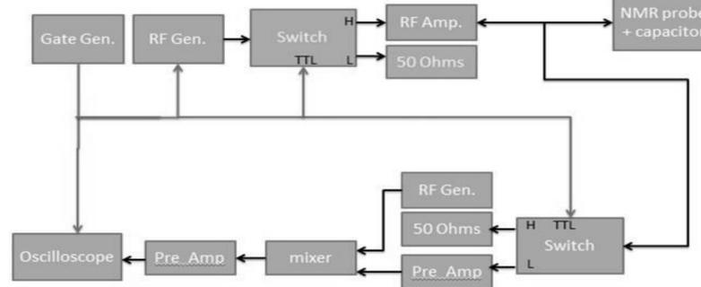
Figure 5. Design of the Pulse NMR system [4]
