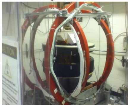
Figure 3. The target cell apparatus with Helmholtz and RF coils
