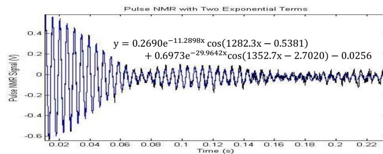
Figure 6. Pulse NMR data in black and fitting in blue
