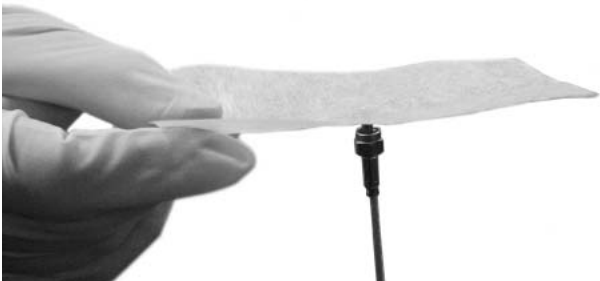
Figure 6-4. Placement of the Optical Fiber Against the Lens Tissue
