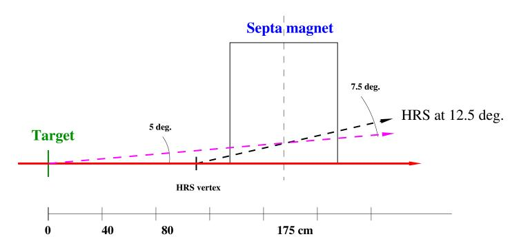
Septa works well for  $\Delta p/p << 1$ . In HRS  $\Delta p/p$  is of 0.09 Required field integral is 0.44 Tesla-m per 1 GeV/c APEX is approved to run with 1.1, 2.2, 3.3, and 4.4 GeV beam energies, which requires 0.55, 1.1, 1.65, and 2.2 GeV in HRS
