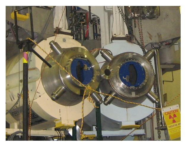
Limited space between Q1s for the beam line pipe Minimum angle for HRS is 12.5 degrees
