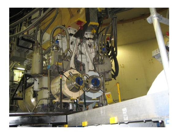
Combined field of Q1s, Q2s, Dipoles on the beam line requires attention Limiting aperture of the beam line for upstream target causes add. radiation
