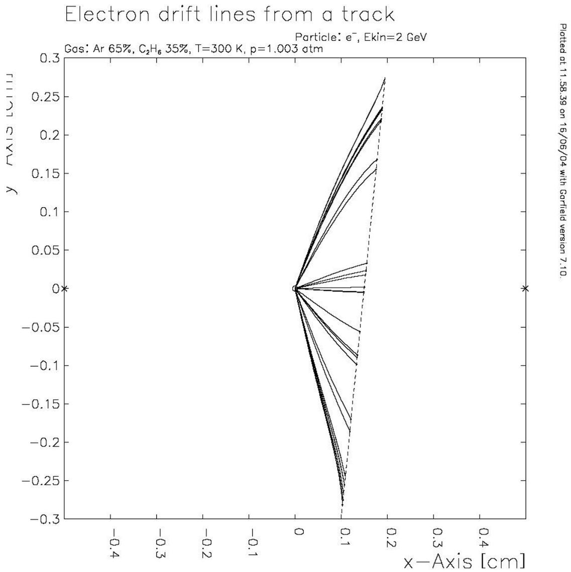
Figure 8: GARFIELD simulation of a 2 GeV electron track going through a plane of the BigBite drift chamber
