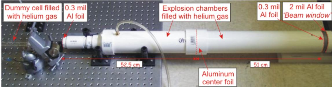
Five new dummy cells were ordered for this test round. The gas inlet of cell # 4 broke during its installation. Furthermore, it turned out to be difficult to cause cell # 3 to rupture. In the end this one and the three other dummies exploded catastrophically.
