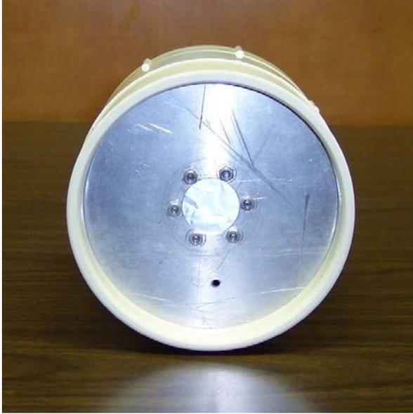
This photo shows the center window foil and frame inside the upstream explosion chamber.
