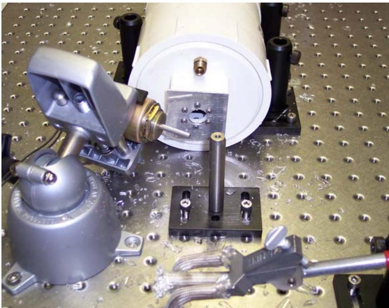
Most of the cells ruptured when the piston hit the cell window the first time. Only two cells did not explode during the first attempt but needed several attempts. All cells exploded catastrophically, means the complete target chamber burst into little pieces as can be seen on the photo on the left. It shows also the frame of the downstream window; the foil was blown out completely.
