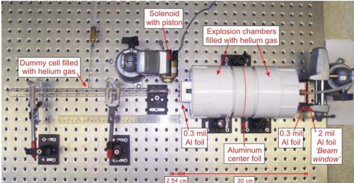
Four dummy cells which were ordered from the same glass blower who produces the cells that are used in Hall A, and one cell that was left over from the rupture tests in 2003, were used in this portion of the test. The results of these five tests can be found in the table on page 4. The pressure that is mentioned is the pressure of the  $^4\text{He}$  gas in the dummy cell. The aluminum foil used as center window had a thickness of 1 mil.
