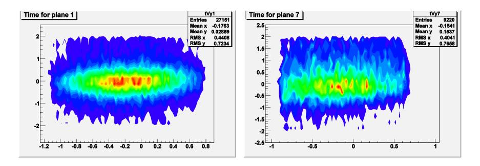
This is for proton events. This is not full statistics nor all selection tools. These diagrams show that there is not a significant systematic y dependence as we look deeper into the neutron detector.
