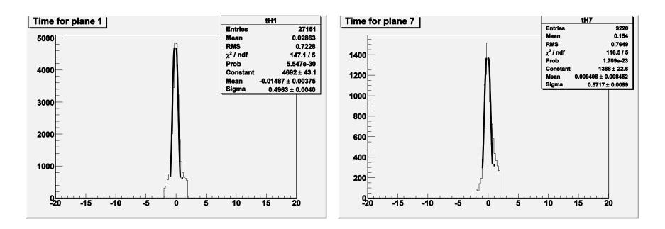
This is for proton events. This is not full statistics nor all selection tools. These diagrams show that the peak does not shift systematically or significantly. The sigma of the distribution is wider, but not significantly so.
