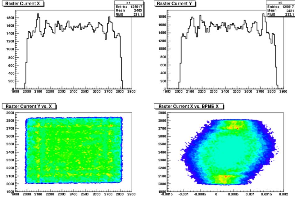
Figure 3: Raster Currents and Raster Current vs. BPM - Run 3356 - Optics Foils, Kin. 3
