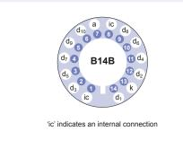
Our range of B14B sockets is available to suit the B14B hardpin base. The socket range includes versions with or without a mounting flange, and versions with contacts for mounting directly onto printed circuit boards.
