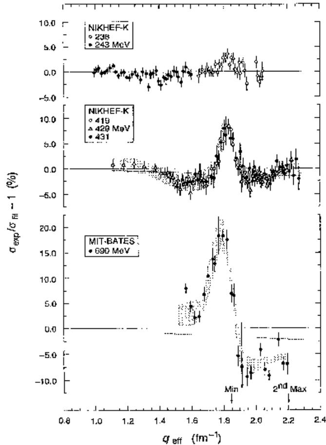
FIG. 11. The differences between the cross sections measured at six incident electron energies (from 238 to 690 MeV) and the values predicted by the ground-state charge density parameters obtained from the data at lower energies (see text). The dashed curves indicate the energy dependence of the dispersive contribution according to Friar and Rosen [12] between 240 MeV and the energy under consideration.
