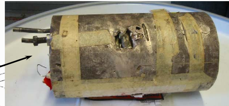
12.5cm dia x 21cm lg silver calorimeter
