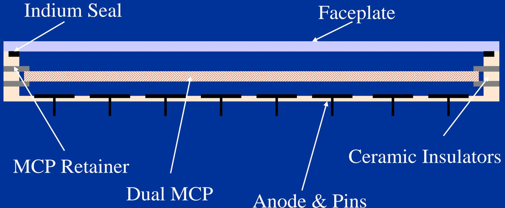
Spacing between faceplate and MCP and MCP and anode can be varied for different applications
