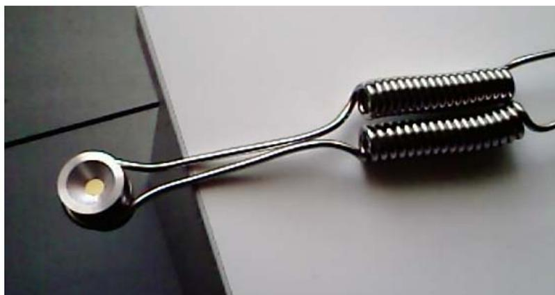
**Figure 9 - Film deposition probe**
