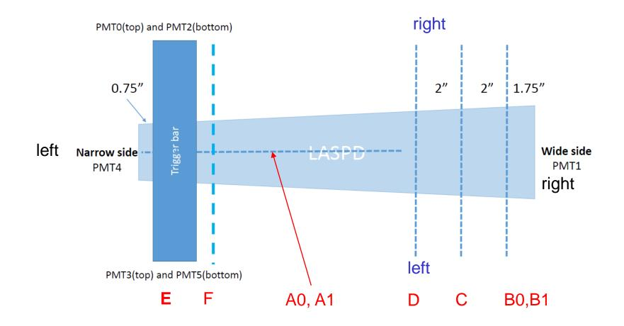
Low HV: A0, B0, C, D High HV: A1, B1, E, F Data set F uses only 2 GEM detectors. All the others use 3 GEM detectors
