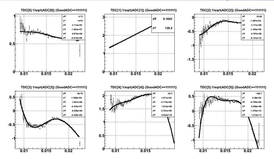
Current calibration is not good at all. Will use the above fit do do 2<sup>nd</sup> order calibration.
