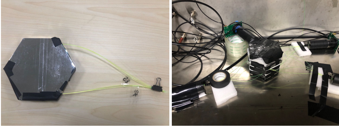
Figure 6: Left: Preshower with fiber wrapped by ESR. Right: Preshower test setup in light-tight box. 4 preshowers are stacked together in the center of picture.
