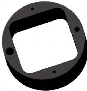
Figure 4: Schematic view of a MAPMT support.
