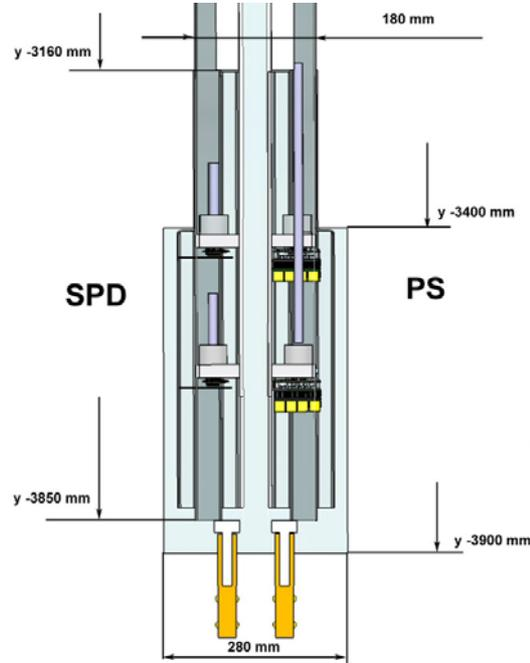
Figure 12: Schematic view of the PS/SPD envelop.
