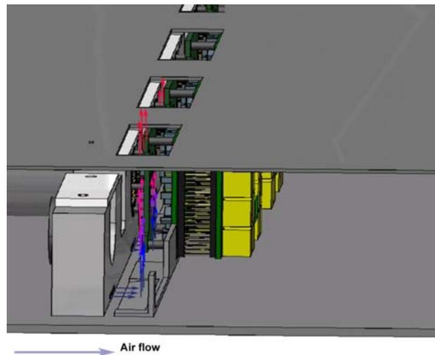
Figure 14: Schematic view of the cooling inside a box.
