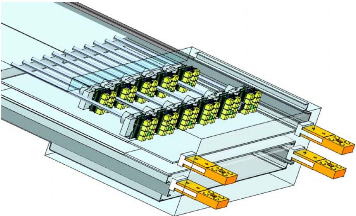
Figure 17: Schematic view of a MAPMT box.
