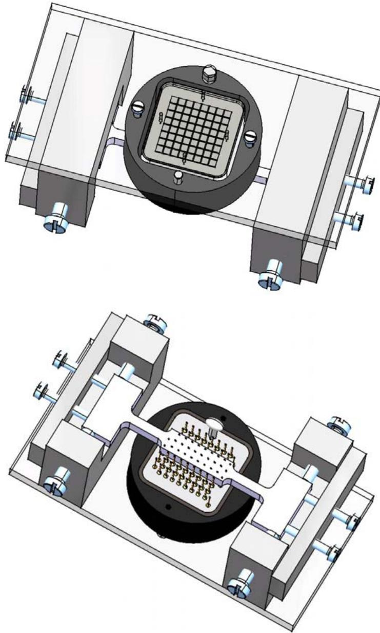
Figure 6: Drawings of the setting tool to position the MAPMT in its support; top and bottom view.
