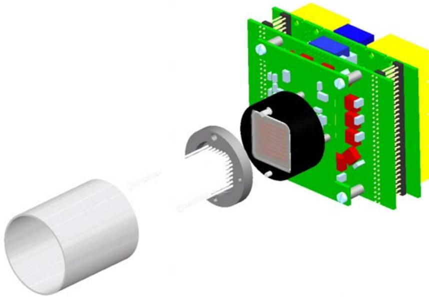
Figure 16: Schematic view of the MAPMT block assembly.
