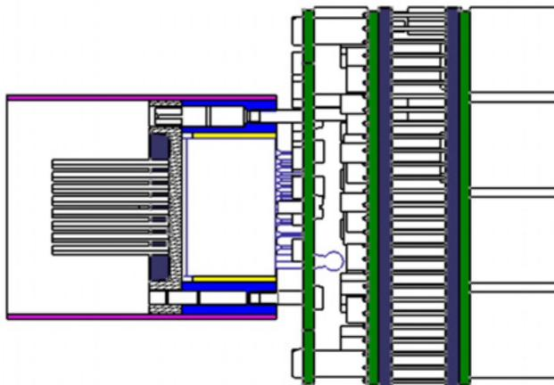
Figure 8: Schematic view of the magnetic shielding in  $\mu$  metal (section view).
