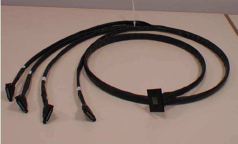
Figure 2: Picture of a fiber strand with the connectors (the MAPMT mask is an old design).
