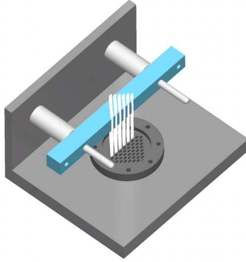
Figure 7: Drawing of the tool to position and maintain the 128 fibres into a MAPMT mask.
