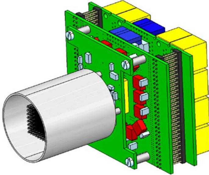
Figure 9: Schematic view of a MAPMT block. The dimension of the PS VFE board is  $72 \times 110 \text{ mm}^2$ .
