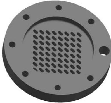
Figure 3: Schematic view of a MAPMT mask.
