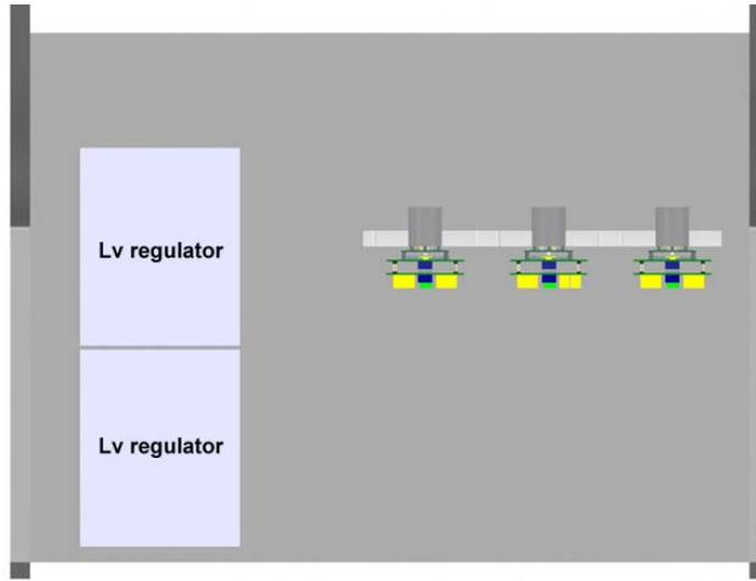
Figure 11: Schematic view of the regulators location inside a MAPMT box.
