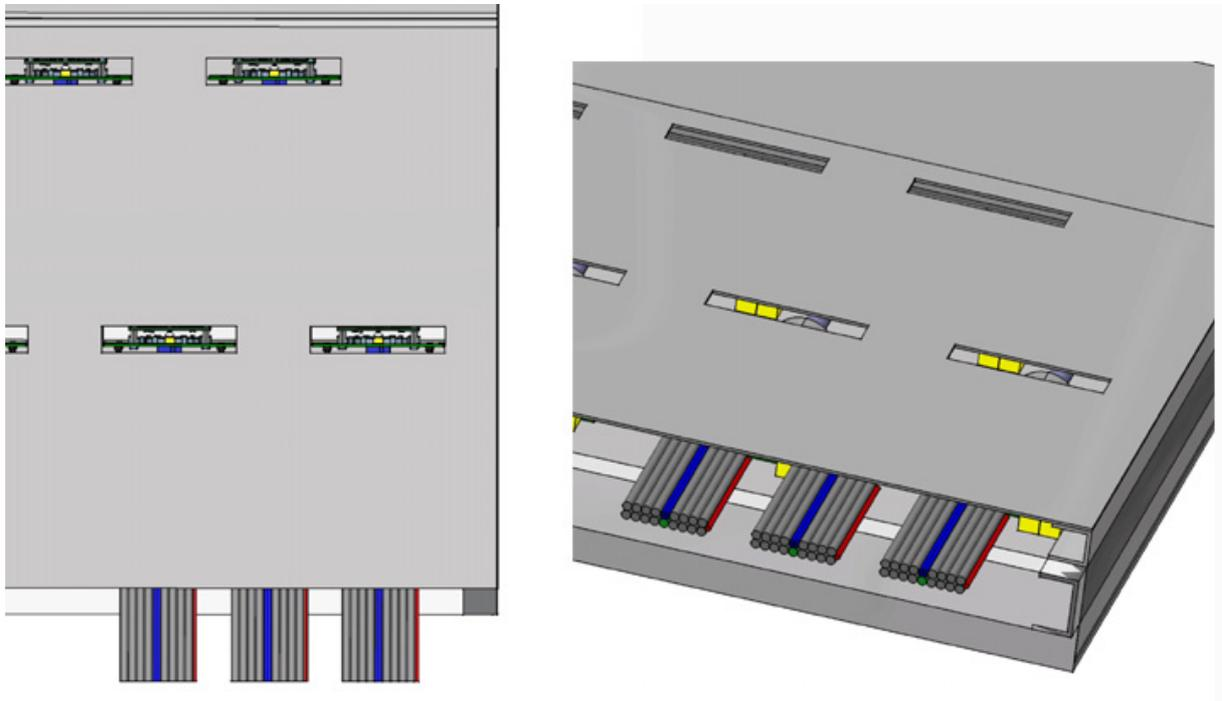
Figure 18: Schematic view of the cable disposition to go out the MAPMT box.
