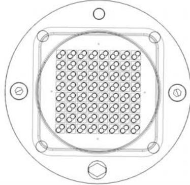
Figure 5: MAPMT anodes position in front the fibre mask inside its support.
