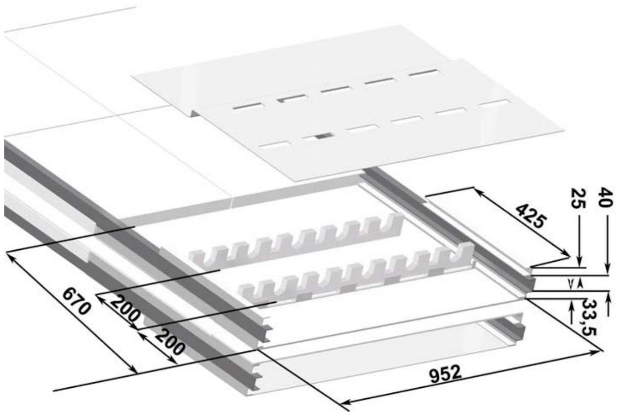
Figure 10: Schematic view of a MAPMT box, with MAPMT supports and its cover, attached to a supermodule (dimensions are in mm).
