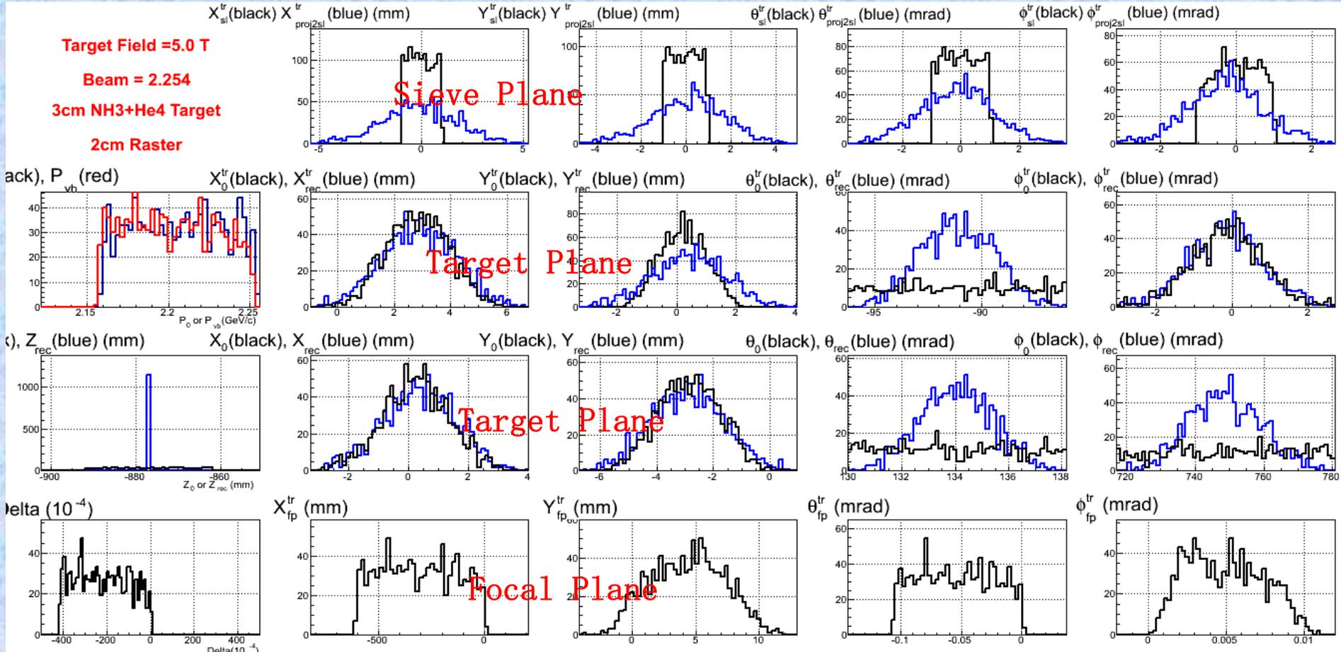
Select 4-D bins in the Sieve Plane, look at the distribution of  $x$ ,  $\theta$ ,  $y$ ,  $\phi$  at the Target Plane
