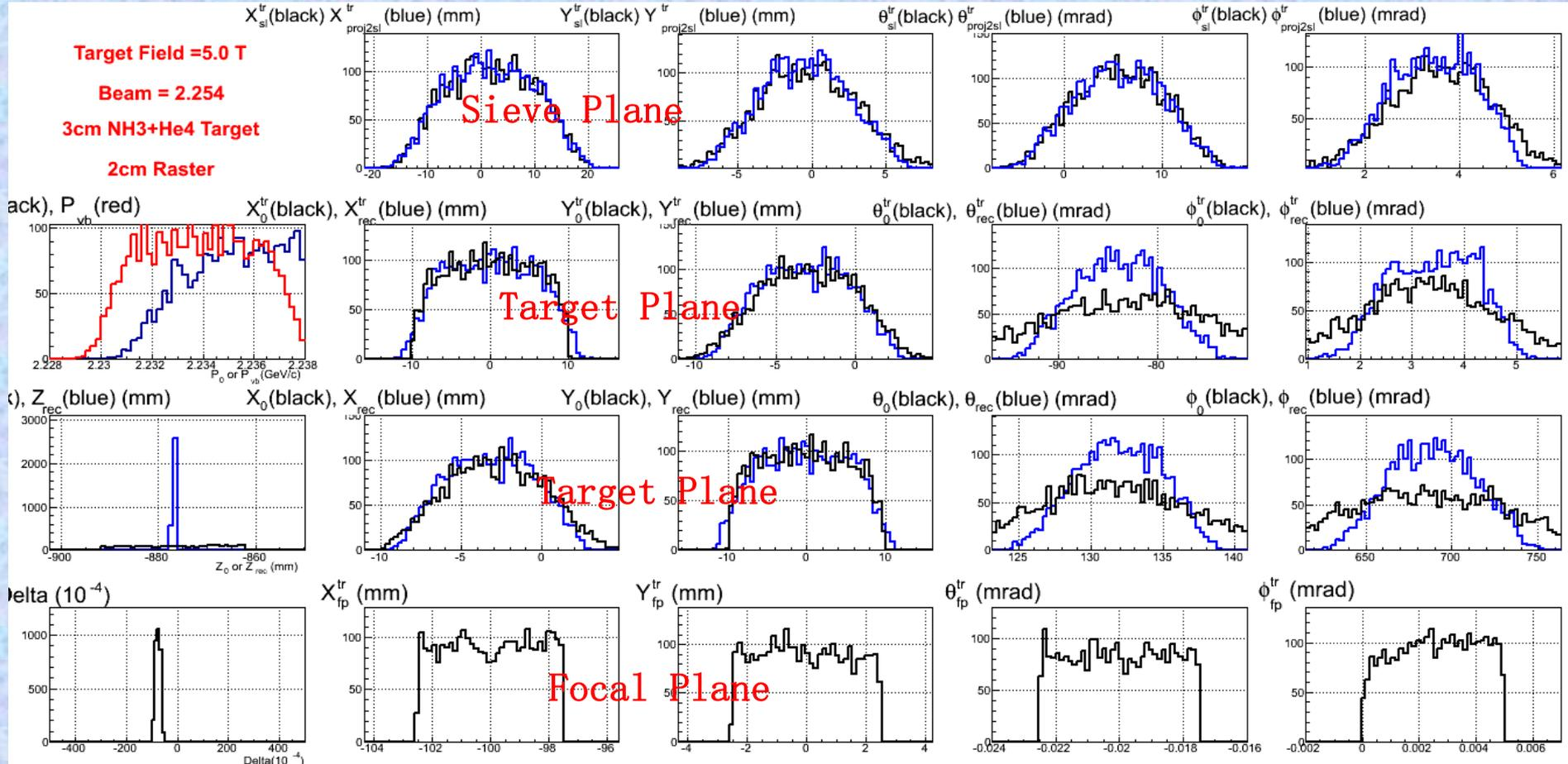
Select 4-D bins in the Focal Plane, look at the distribution of  $x$ ,  $\theta$ ,  $y$ ,  $\phi$  at the Target Plane
