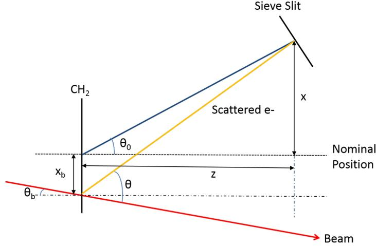
Figure 1: Schematic of the angle measurement on CH<sub>2</sub> foil target.
