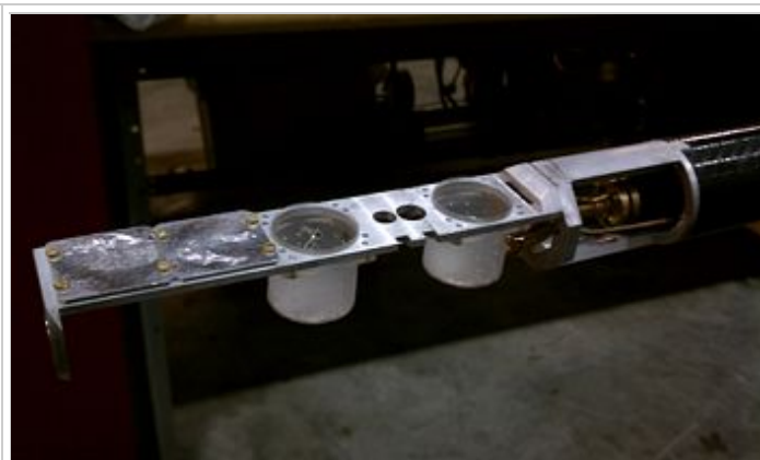
Ladder of new inserts, with two target cups, NMR coils and microwave horn.
