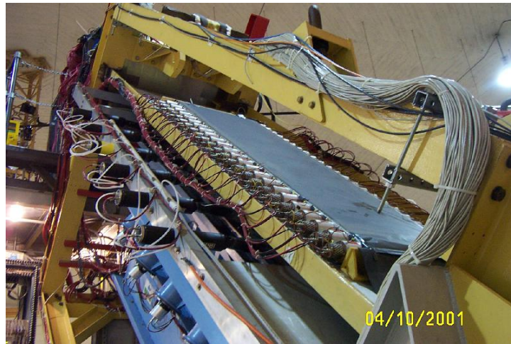
Figure 20.2: HRS-R first layer (“pre-shower”) detector installed, while the second layer (“shower”) detector was removed.
