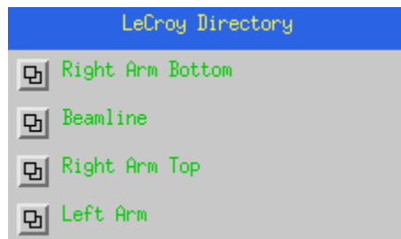
Figure 6.2: Epics Menu for the LeCroy High Voltage supplies in Hall A. All slots related to the eP system can be accessed from the Beamline button.
