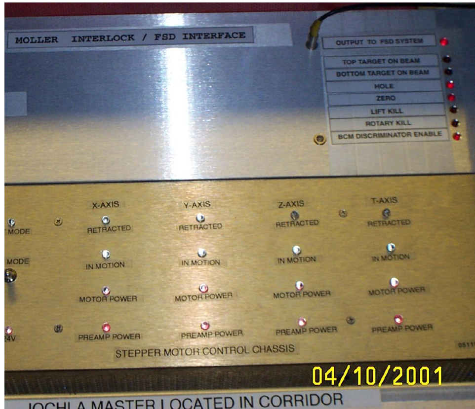
Figure 8.5: The Møller target motion may cause the Fast ShutDown (FSD) of the accelerator. The LEDs in the top right corner show the appropriate signals from the target. The top LED lit indicates no FSD signal.
