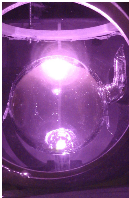
Figure 4-8: Top: schematic diagram of the optics setup for the vertical pumping laser line. Bottom right: photo of the polarizer (for vertical polarization, identical to that for transverse) from a similar viewing angle as the top diagram. Bottom left: photo of the pumping chamber of cell Astral under a vertical laser beam coming from the top. The magenta color of the infrared laser light was due to the imperfect infrared filtering of the camera (Canon SD 700SI).
