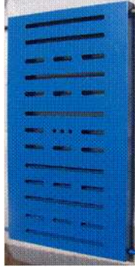
Figure 5.8: A lead sieve slit plate with a thickness of 1.5".
