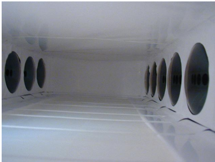
Figure 17.8: Aerogel A1 detector from inside of the diffusion box.
