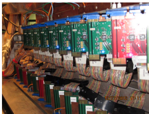
Figure 14.5: The new MAD card that is used as pre-amp/discriminator on VDC. It operates with +5.0 V
