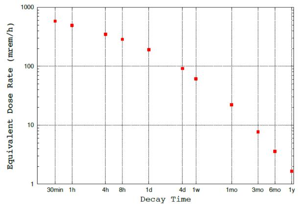
Figure 3: Expected equivalent dose rates at 30 cm from the 0.053  $X_0$  tungsten target after 170 hours of irradiation with 3.3-GeV, 120- $\mu$ A beam followed by 314 hours of irradiation with 4.4-GeV, 90- $\mu$ A beam.
