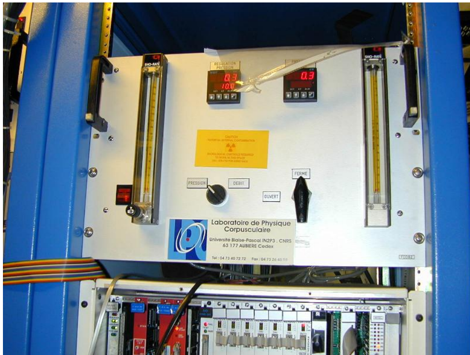
Figure 6.15: Picture of the gas controller of the eP gas Cherenkov detectors.
