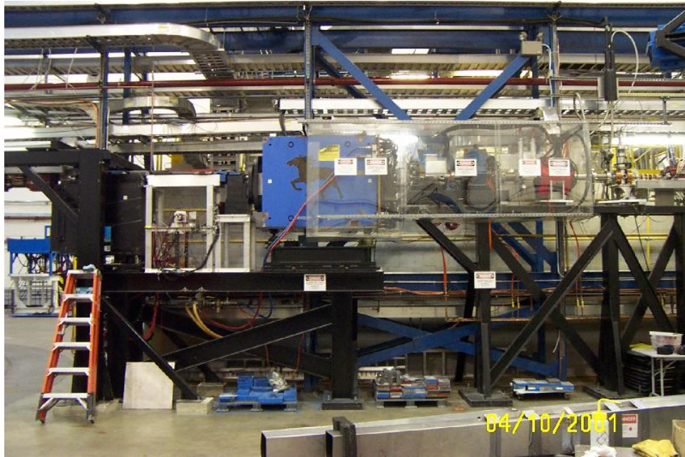
Figure 8.8: The Møller spectrometer. The target is located at the right side of the photograph, the blue dipole magnet is close to the center.
