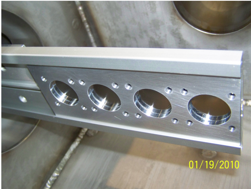
Figure 8.7: The Møller target holder. It carries four ferromagnetic foils, stretched at 90^\circ to the beam. The beam comes from the bottom of the picture.
