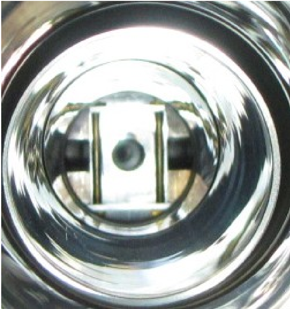
Figure 8.9: The Møller dipole collimator is located in front of the dipole. The Møller electrons pass through right and left slits of the collimator. The electron beam passes through the collimator in the center.
