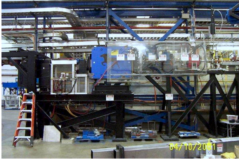
Figure 8.6: The Møller spectrometer. The target is located at the right side of the photograph, the blue dipole magnet is close to the center.
