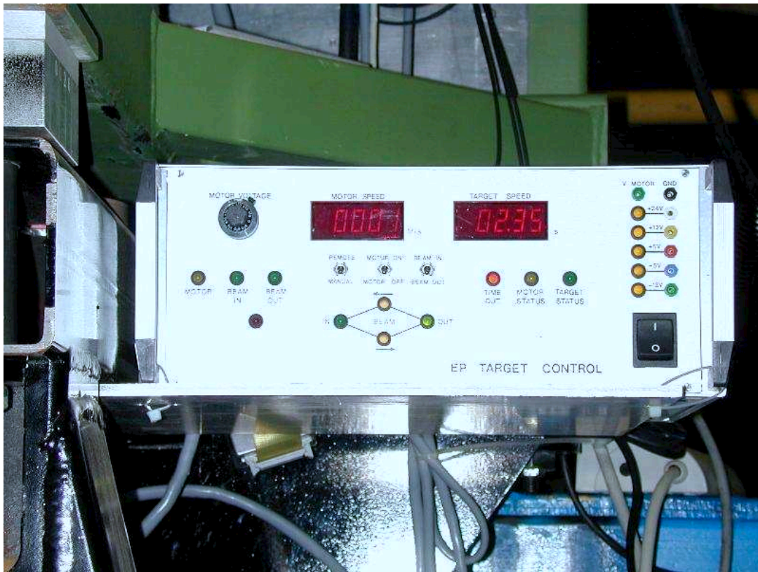
Figure 6.12: Control box for the eP target system.
