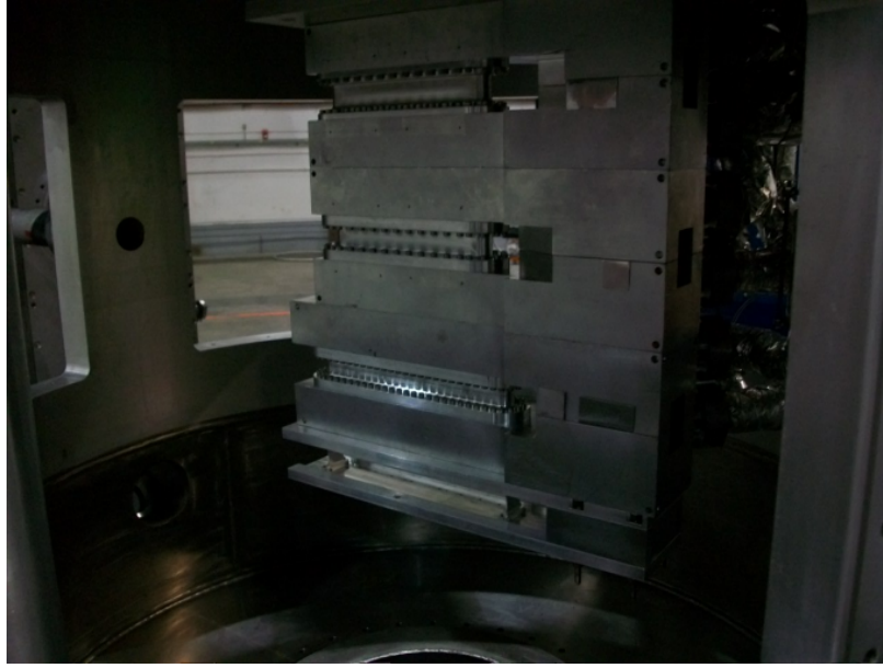
Figure 2.8: Picture of the cryogenic target ladder inside the scattering chamber.
