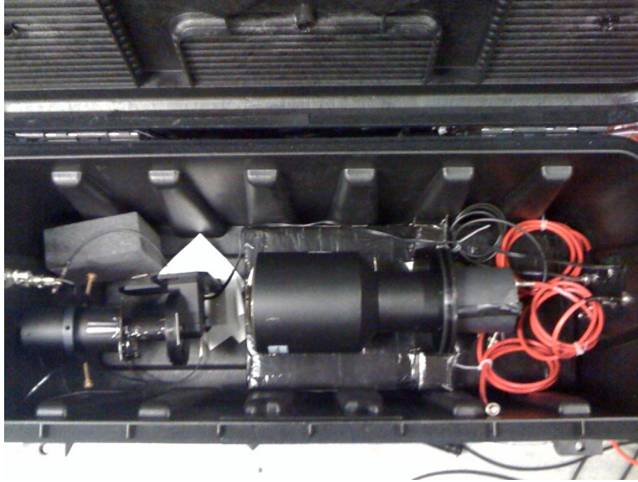
Figure 3.18: Picture of the linearity test experimental setup. PMT shown was 5-inch Burle used in HAPPEX-III.
