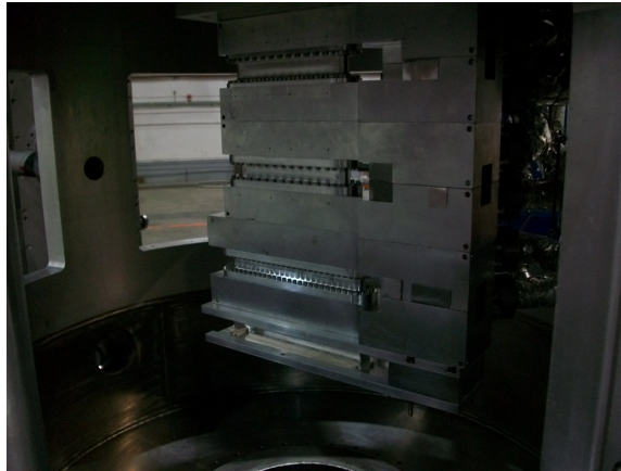
Figure 3.6.2: HAPPEX-III used cryogenic liquid-hydrogen (LH 2 ) targets contained in a race-track shaped aluminum (Al) cells. The target ladder contained three such cells, but only two were used during HAPPEX-III. The bottom cell on loop 3 (L3) was 25 cm long, and the top two cells on loops 1 (L1) and 2 (L2) were each 20 cm long. The L3 cell was used for majority of the run, until it malfunctioned due to a power outage. Then, HAPPEX-III ran with the L1 cell for about 1 week before the end of the experiment. The electron beam propagated into the scattering chamber through the hole towards the center and to the left of the target above.
