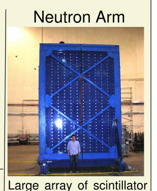
with over 500 PMTs and active area of about 10m<sup>2</sup> provides detection of recoiling nucleons.
