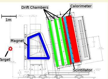
BigBite is a large angular and momentum acceptance spectrometer consisting of a large dipole magnet with a solid angle of 100 msr and associated detector
